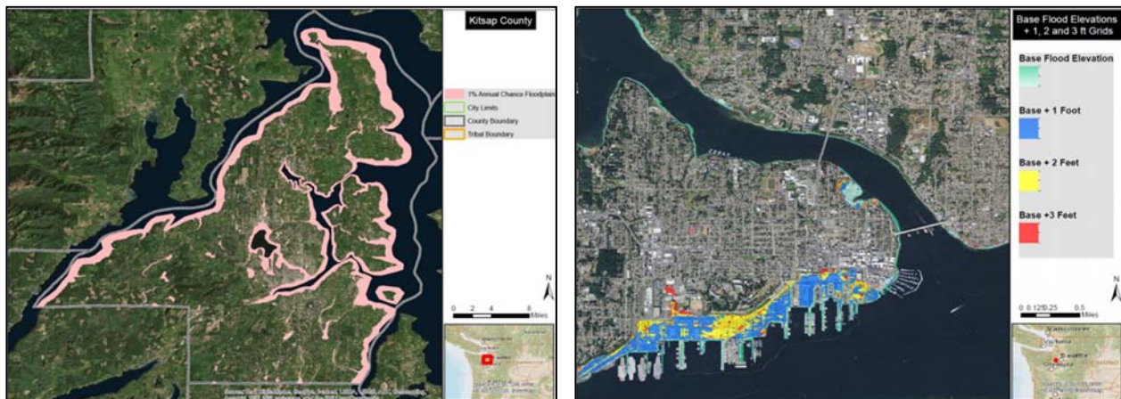
Figure 49. 1% Annual Change Floodplains for Kitsap County (left); Future Risk if Flooding Occurs at 1 Foot, 2 Feet, and 3 Feet for Bremerton (right) 705
