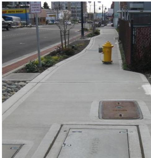
The hydrant is in the sidewalk and located towards the outside edge. The remaining clear width of the sidewalk meets ADA requirements. Other new fire hydrants installed on Pacific Avenue and elsewhere in the downtown from recent projects are not in the far side of the sidewalks and are closer to the curb. While this may meet ADA standards, it is not a logical placement.
