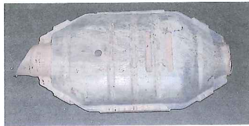
Catalytic Converter Unit
